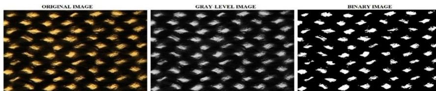
Fig. 3: Steps of image analysis for fabric porosity
