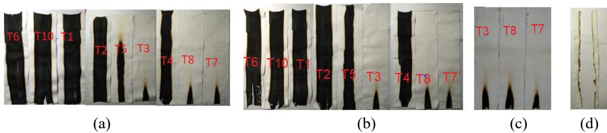
Fig. 1. Vertical flammability of, (a) After treatment, (b) after 10 of washing cycles, (c) After 30 of washing cycles, and (d) control
