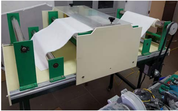
Fig. 1. DBD plasma reactor
