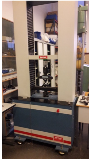
Figure 4. Universal Testing Machine used for flexural tests
