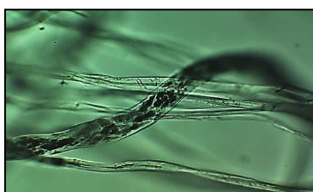
Figure 2. Optical microscope view of the cotton fibres and also the regenerated cellulose with Ag + ions fibre at 400x magnification
