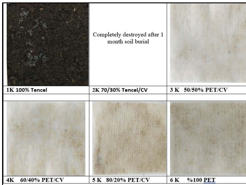
Figure 2. The test samples after two months soil burial period
