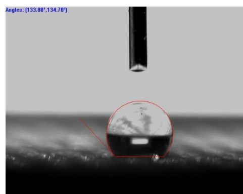
Figure 5. Photo of water droplet on the cotton fabric
