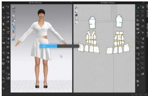
Figure 8. Product simulation- checking the distribution of the fullness
