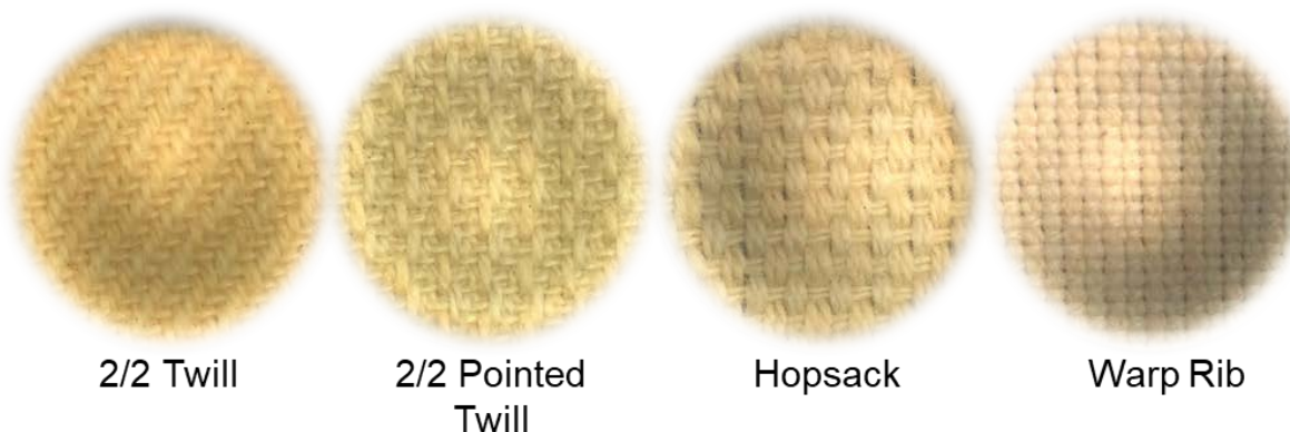
Figure 1. The appearance of the 4 types of used weave patterns
