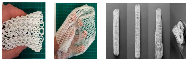
Figure 6. 3D knits obtained through a 3D printing technique [8]
