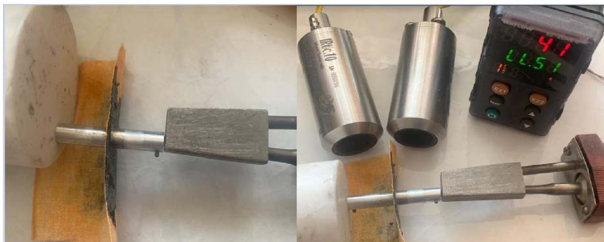
Figure 5. Rubber-textile composite material heat transfer measurement
