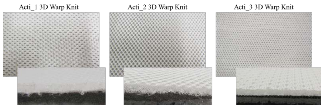
Figure 1. Representative images of the warp-knit spacer surface and connection structures
