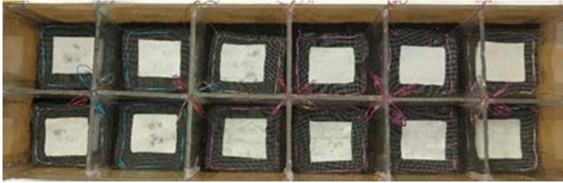
Figure 1. The test samples in plexiglass boxes for soil burial test
